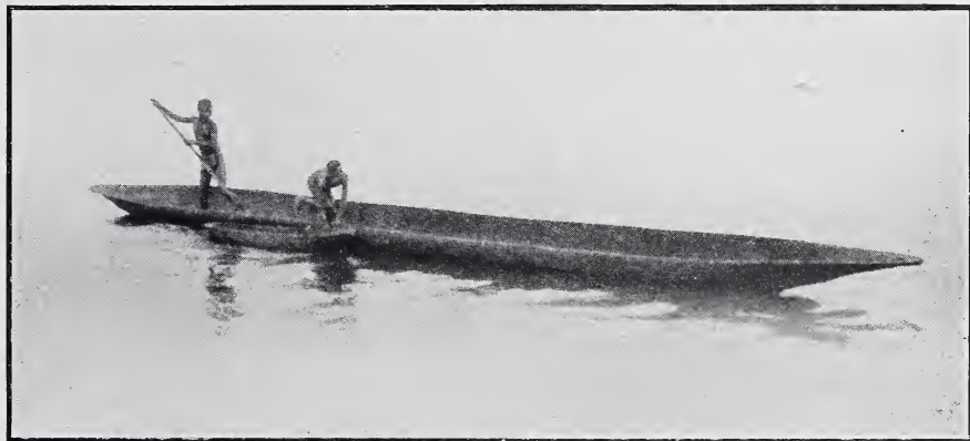
Native canoes along the Congo River are but hollowed logs. They range in size from the small, one-man canoe to the long ones which will accommodate from twelve to twenty natives.
